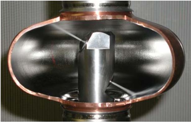
Figure 8: Test of the dry-ice nozzle system in a cut NbCu-cavity
