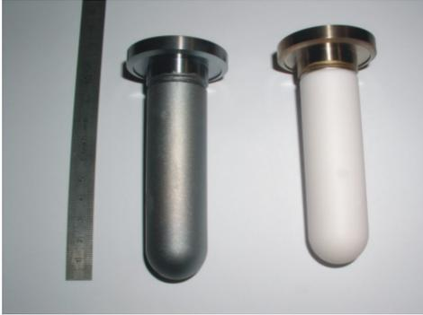
Figure 3: Cold alumina window before (right) and after Ge plating
