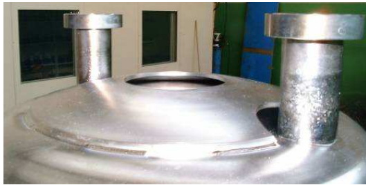
Figure 6: \beta=0.12 torus stiffener
