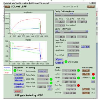
Figure 1. Low Level RF traces of forward (blue) reflected (green) and transmitted (red) amplitude (above) and phase (below) for a SNS superconducting cavity in open loop. Data acquisition terminates 50 µsec after the end of the RF pulse
