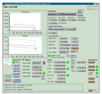
Figure 2. Low Level RF screen showing the RF amplitudes (Forward blue, transmitted red, reflected green) during a quench event for an SNS superconducting cavity. During the quench the loaded Q drops to about  $3x10^5$  and the unloaded  $Q_0$  to  $4x10^5$ .
