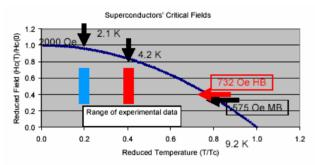
Figure 4. Theoretical magnetic field limits for a superconductor as a function of temperature. The operating values for SNS are well below the theoretical limits (blue curve). Experimental maximum field ranges are essentially identical at 4.2 K (red bar) and at 2.1 K (blue bar).
