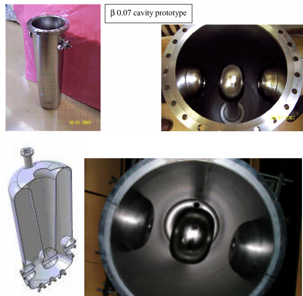
Figure 6: Low (up) and high (down) beta cavities
