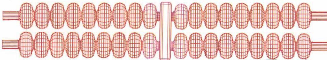
Figure 2: An example of single cell coupled multi-cell two-beam structures.
