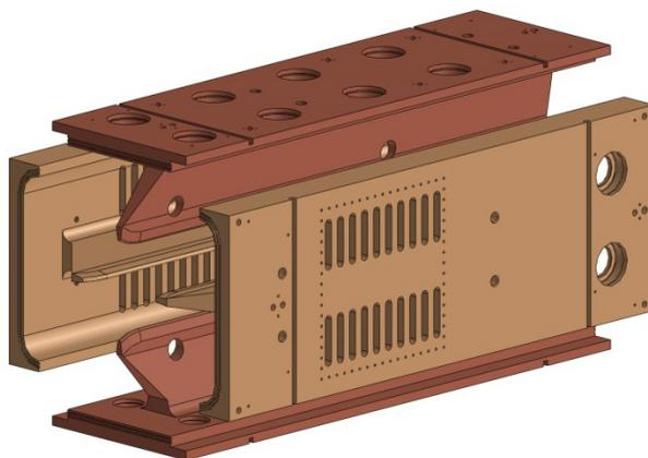
Figure 2: Exploded CAD model of four machined vane.
