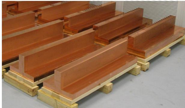
Figure 1: Raw tee shaped copper for vane fabrication.
