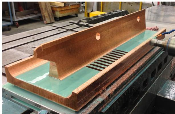
Figure 3: Module 1, horizontal vane being machined.
