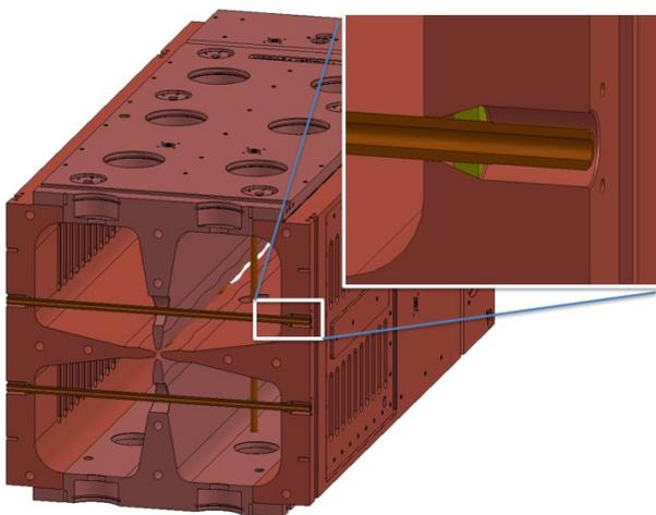
Figure 6: Pi-mode rod with ferrule detail.
