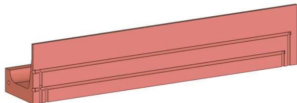
Figure 8: CAD model of gun drilled cooling passages.
