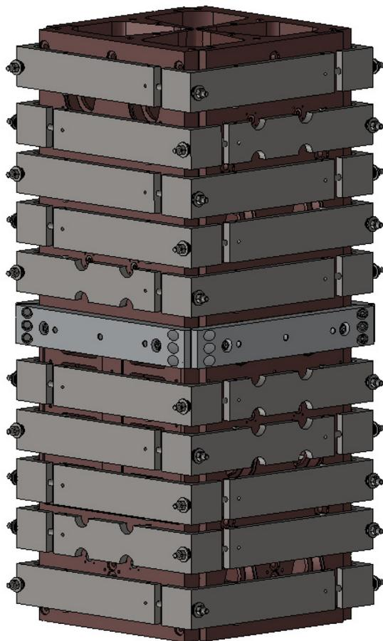
Figure 9: CAD model of vertical module braze with clamps.
