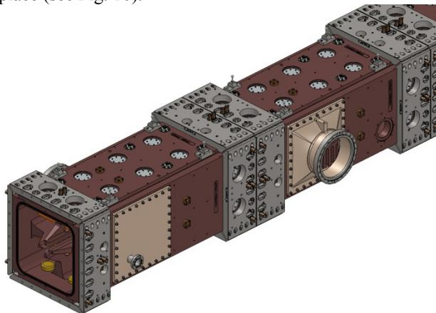
Figure 10: Joint Plates connecting modules.
