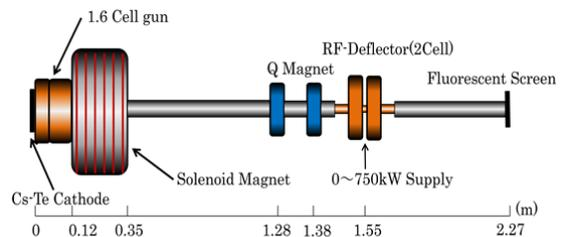
Figure 8: Setup of rf-deflector system.
