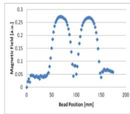
Figure 5: Magnetic field in 2 cell rf-deflector.
