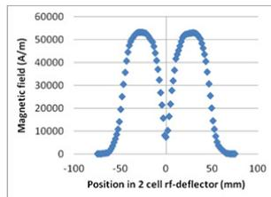
Figure 3: Magnetic field in 2 cell rf-deflector with 750 kW supply (HFSS).
