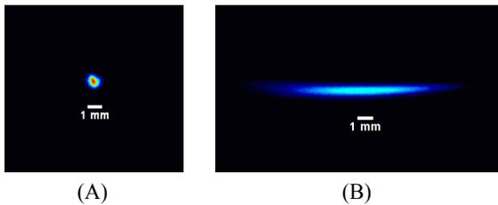
Figure 10: Observed beam profiles. (A): deflector is off, (B): deflected bunch at the zero-crossing phase.
