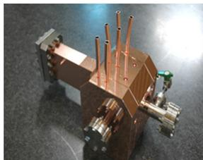
Figure 4: Structure of 2 cell rf-deflector.
