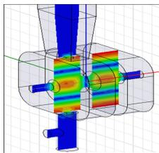
Figure 2: Structure of 2 cell rf-deflector (HFSS).
