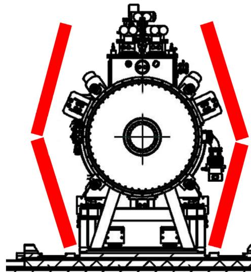
Figure 2: General Concept, frontal view. The partial return yoke is shown schematically in red.
