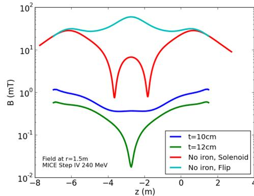
Figure 3: Modulus of the magnetic fringe field at a radius of 1.5 m at beam height.
