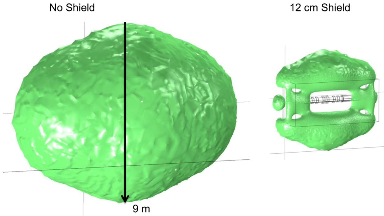
Figure 4: 5 Gauss iso-surface plot of MICE for the 200 MeV flip mode. The left figure shows the 5 Gauss surface for an unshielded scenario (no iron present) versus the case where the PRY is adopted.
