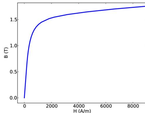
Figure 1: Magnetization curve of AISI 1010 steel.
