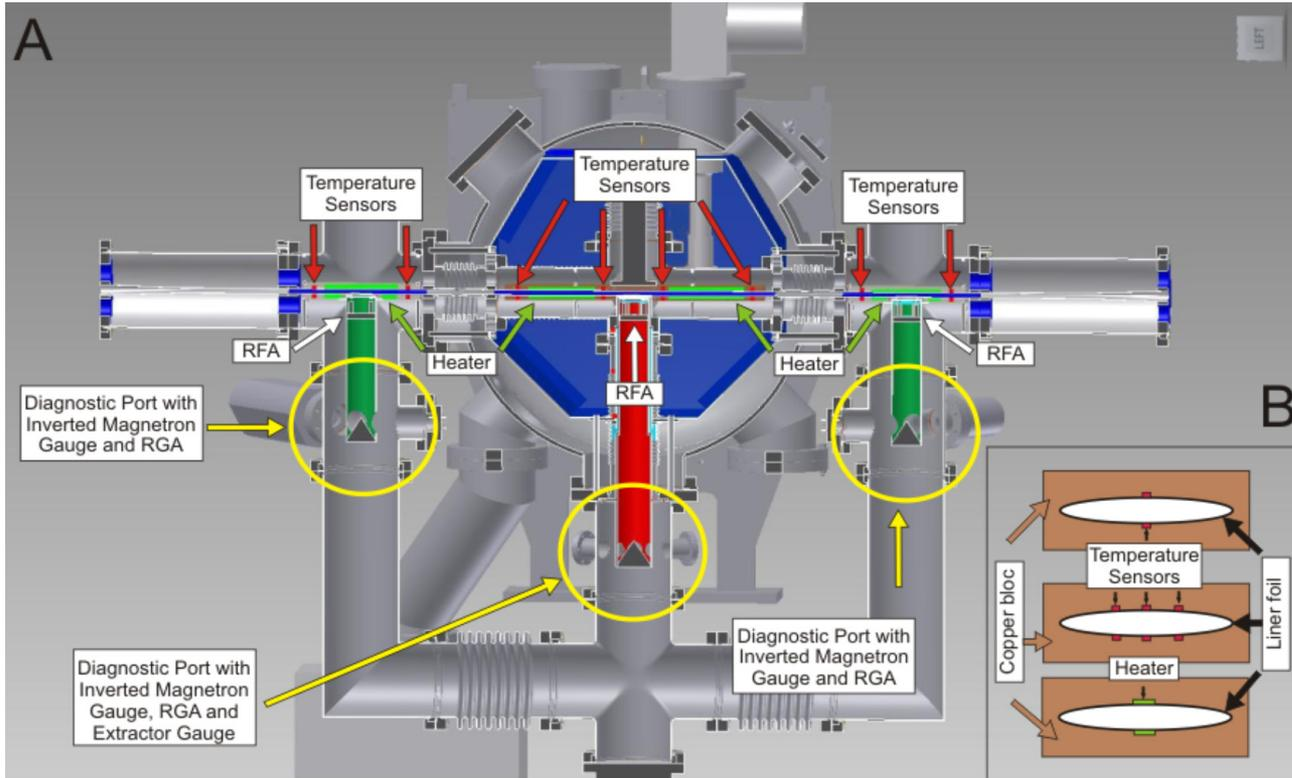
The diagnostics will include measurements of the heat load, the pressure, the gas composition, and the electron flux of the electrons bombarding the wall.
