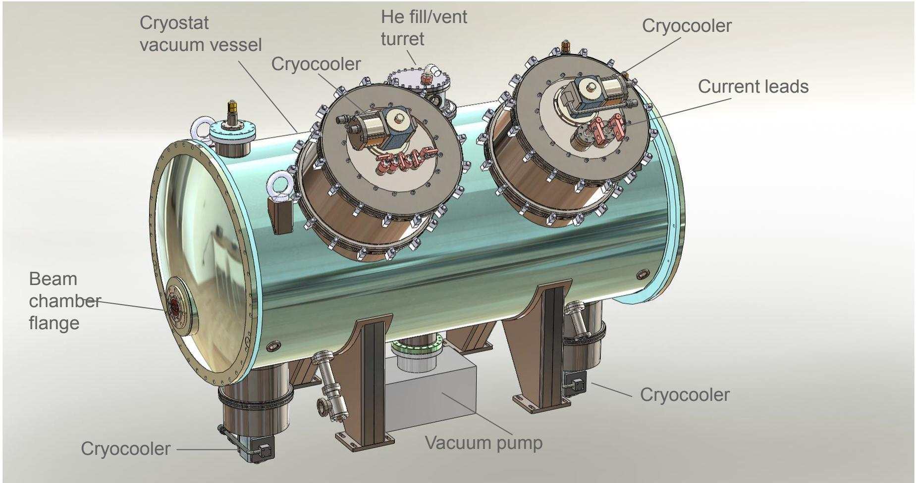
Cryostat is 2.06 m long, so will fit in half of the straight section
