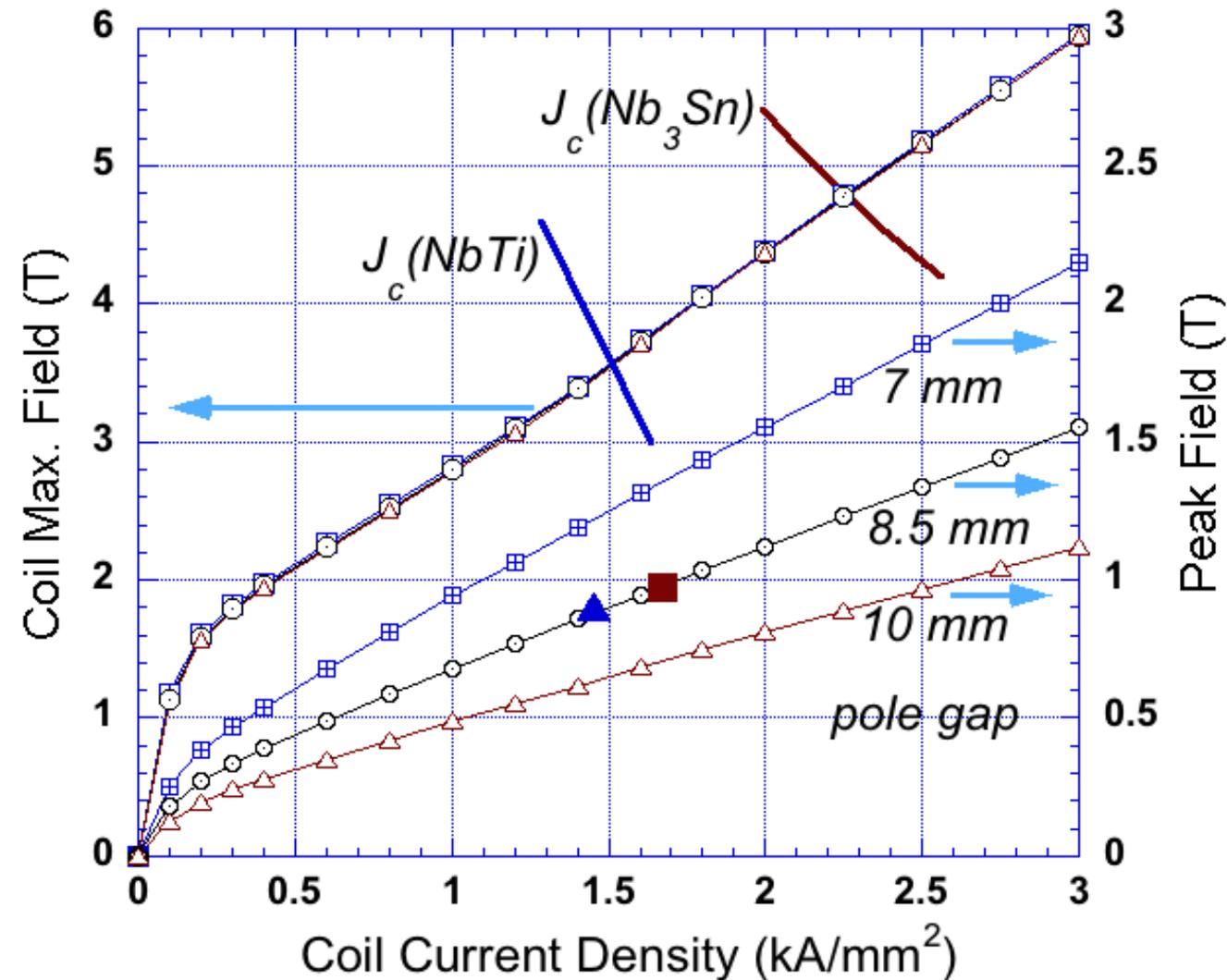
Calculated peak on-axis field (*right*) and max field in the coil (*left*) as a function of average current density in the coil for pole gaps of 7, 8.5, and 10 mm.
