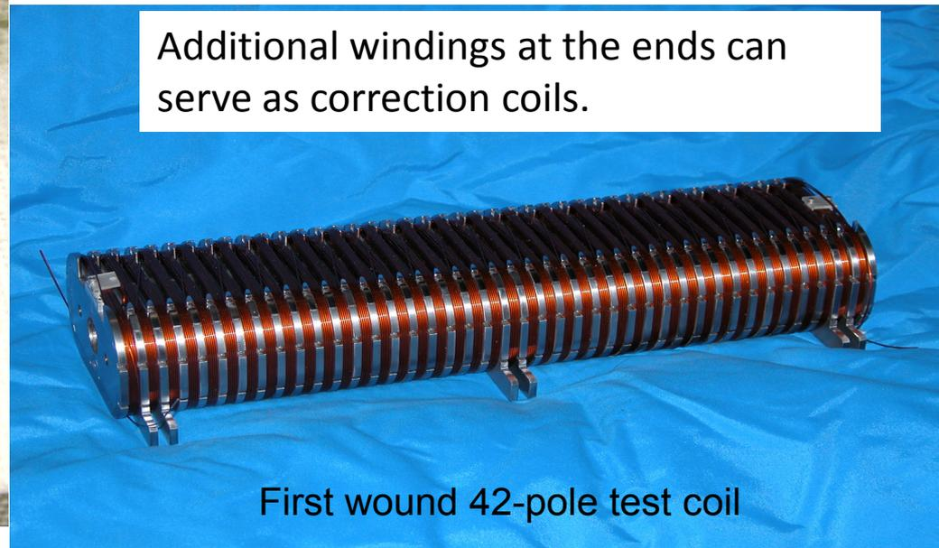
Additional windings at the ends can serve as correction coils.
