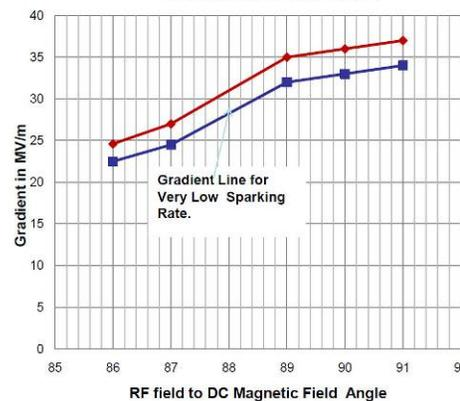
Operated stably at 50 MV/m at  $B = 0$  but only 35 MV/m at 3 T
