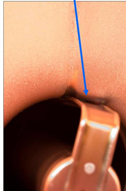
Cu deposition on TiN coated ceramic RF window
