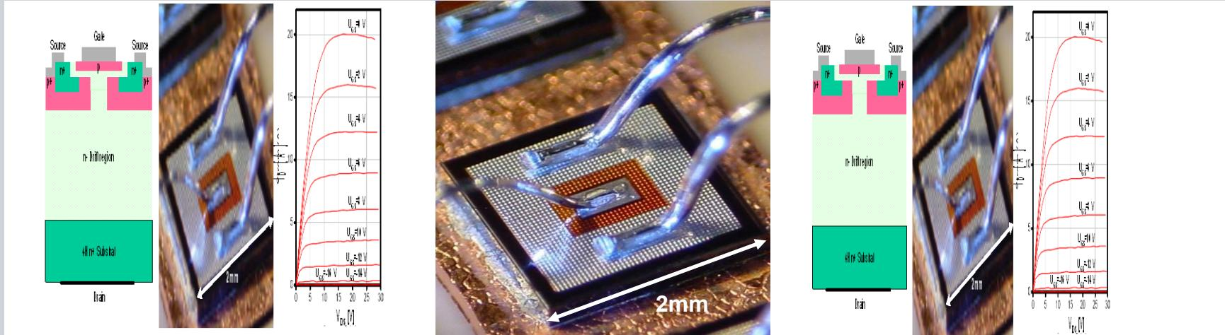
Normally on vertical junction FET (vJFET) with intrinsic body diode
