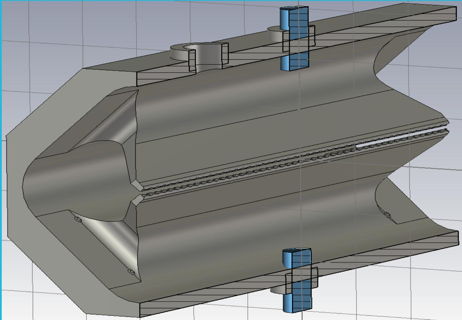
**Low Level RF control system, cold model** to be built in Aluminum.
