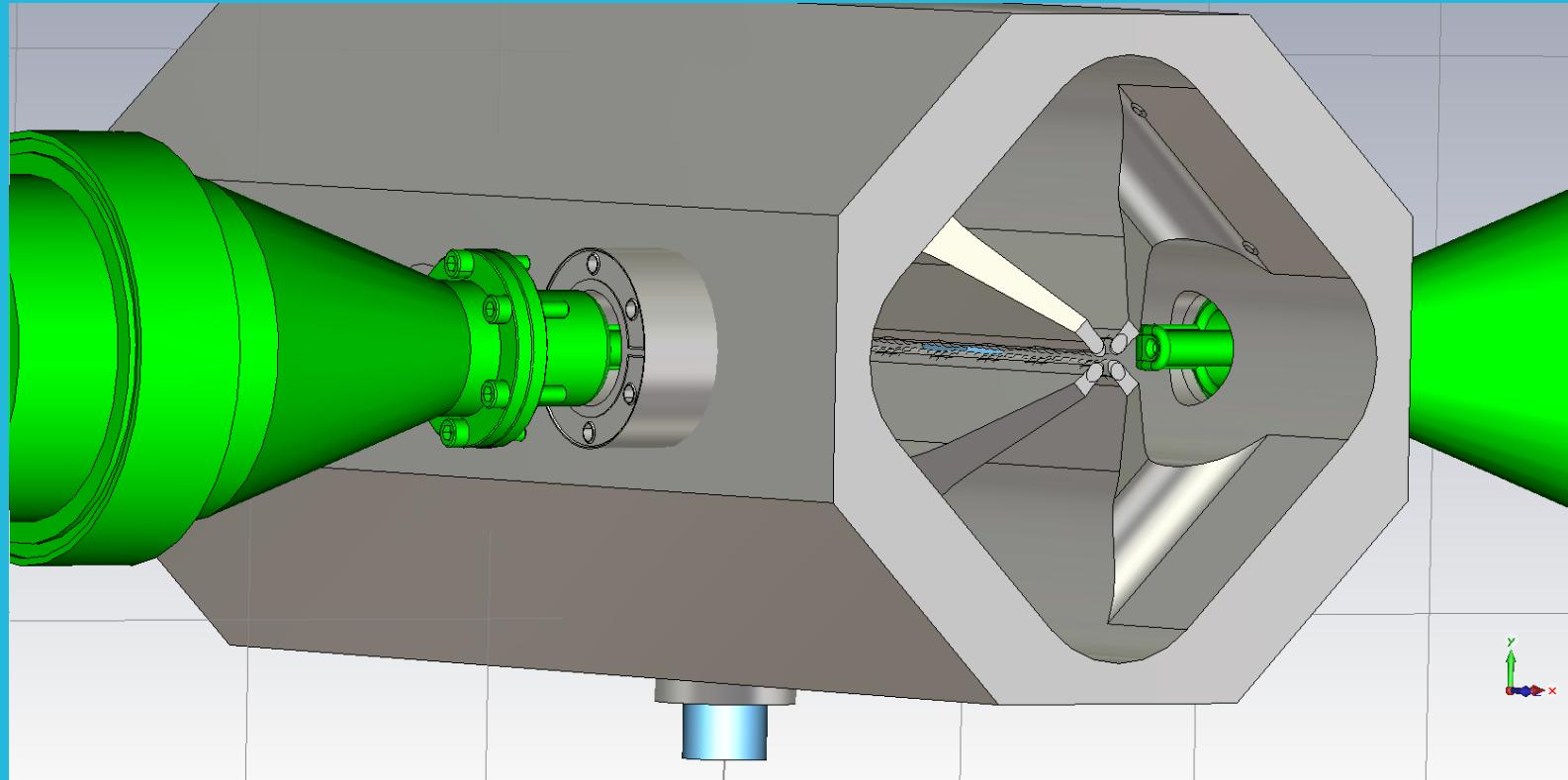
Cavity design: **couplers** and **tuners** positions
