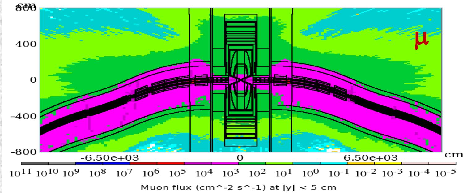
Dipoles close to the IP and tungsten masks in each interconnect region help reduce background particle fluxes in the detector by a substantial factor. The tungsten nozzles, assisted by the detector solenoid field, trap most of the decay electrons created close to the IP as well as most of incoherent  $e^+e^-$  pairs generated in the IP. With additional MDI shielding, total reduction of background loads by more than three orders of magnitude is obtained.
