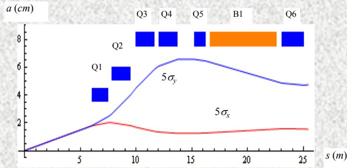
First 4 quadrupoles are operationally stable, while the level in next three IR quadrupoles is 5 to 10 times above the limit. This heat load could be reduced by a tungsten liner in the magnet aperture
