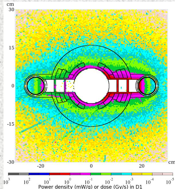
The open midplane design for the dipoles provides for their safe operation. The peak power density in the IR dipoles is about 2.5mW/g, safely below the quench limit for the Nb<sub>3</sub>Sn superconductor based coils at the 1.9-K operation.
