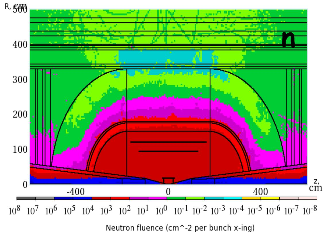
Maximum neutron fluence and absorbed dose in the innermost layer of the silicon tracker for a one-year operation are at a 10% level of that in the LHC detectors at the luminosity of  $10^{34} \text{ cm}^{-2}\text{s}^{-1}$
