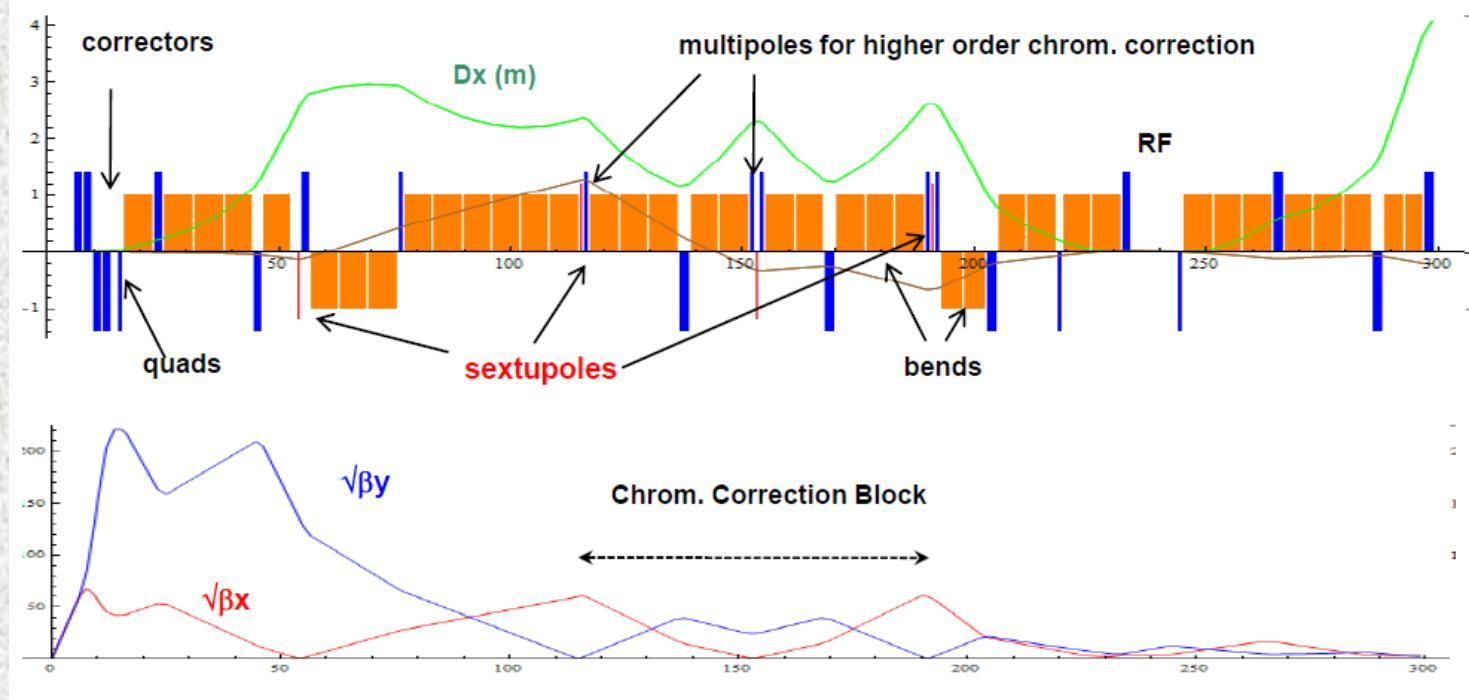
8-T dipoles in IR to generate large D at sextupoles to compensate chromaticity and sweep decay products; momentum acceptance 1.2%; dynamic aperture sufficient for transverse emittance of 50  $\mu\text{m}$ ; under engineering constraints.
