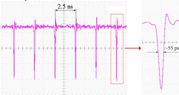
Figure 2: Micro-pulse train of UV laser measured with fast detector.
