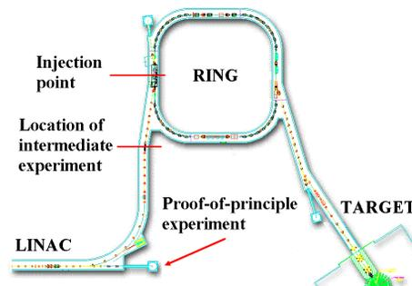
Figure 1: Location of intermediate experiment at the SNS.
