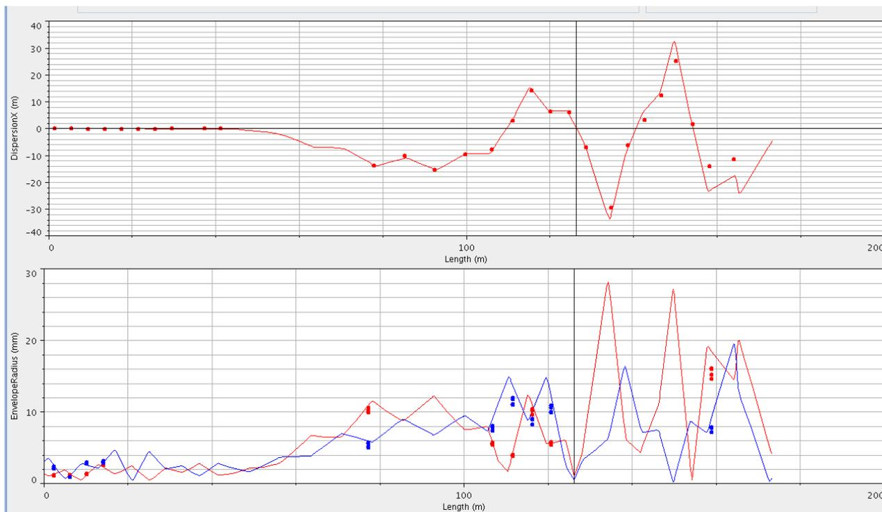
Figure 4: Example of  $H^-$  beam optics setup for laser stripping. The upper plot is a dispersion function. The lower plots are vertical (blue) and horizontal (red) rms transverse envelope radii.
