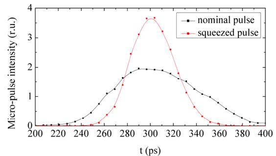
Figure 3: Nominal and squeezed H<sup>-</sup> micro-pulse.
