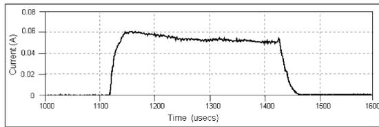
Figure 5: Example of the  $H^-$  current pulse (20mA/div) as measured by the Faraday cup after LEBT.
