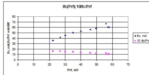
Figure 7: Evolution of the Faraday cup current  $I_{fc}$  and ratio  $I_{fc}/P_{rf}$  as function of  $P_{rf}$  during cesiation. The efficiency of  $I_{fc}$  generation increased with decreased gas flow  $Q$  from 20 sccm to 17.2 sccm.
