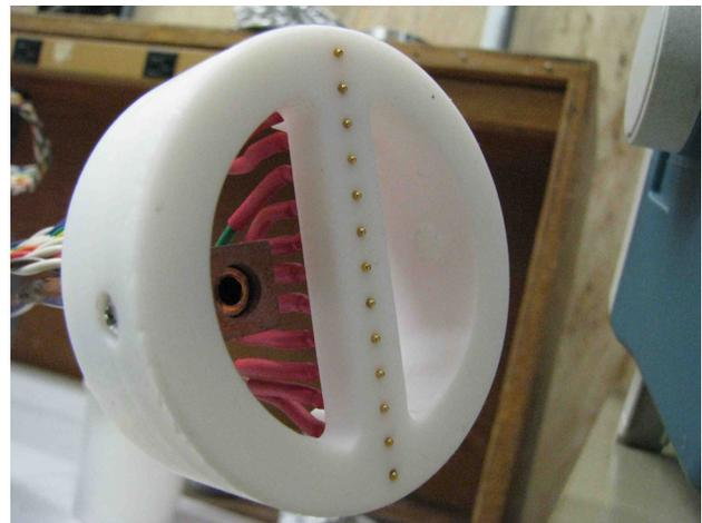
Figure 2: The ion probe with bias voltage can measure the ion current distribution simultaneously for 13 radial positions.
