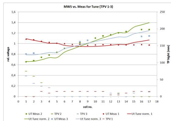
Figure 6: Comparison of Measured Flatness (Dots) for Different Tuning Plate Distributions (Bars) with the Corresponding Results of the Tuning Program (Lines).
