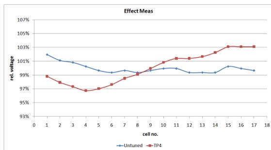
Figure 4: Measured Flatness of the ReA3-RFQ. In Blue the Untuned and in Red the Distribution With a Tuning Plate in Cell No. 4.
