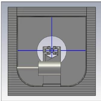
Figure 1: Cross section of the ReA3-RFQ Simulation Model.
