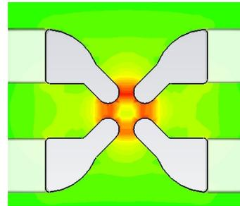
Figure 2: Quadrupole field between electrodes.
