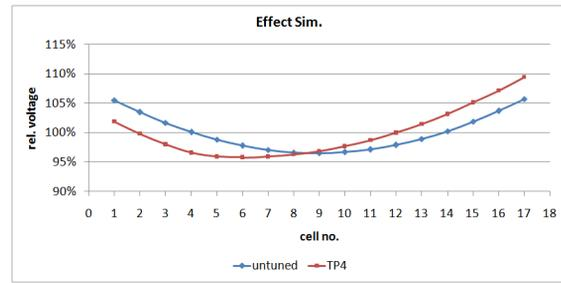
Figure 5: Simulated Flatness of the ReA3-RFQ (Same Case as in Fig. 4).
