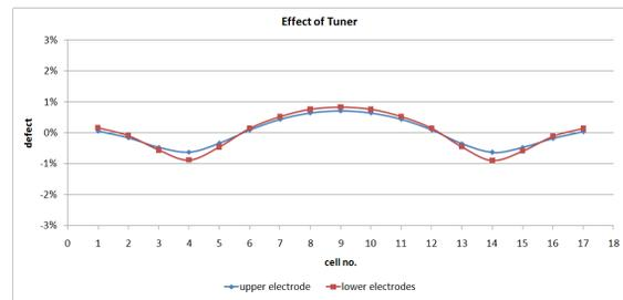
Figure 9: Defect Caused by Piston Tuners.
