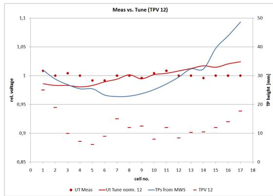
Figure 7: Comparison of the Measurement (Dots) with Results of the Tuning Program (Lines) for the Final Tuning Plate Set Up of the ReA3-RFQ. The Red Distribution is Simulated Based on Measured ECs, While the Blue One Uses Simulated ECs.
