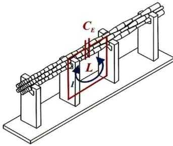
Figure 3: LC Resonator as Equivalent Circuit of a 4-Rod RFQ.
