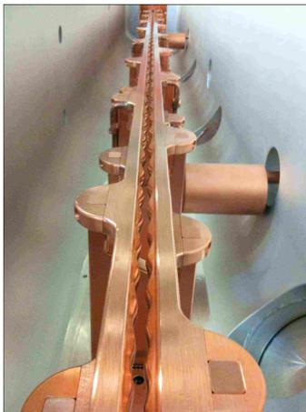
Figure 8: Piston Tuners in ReA3-RFQ.
