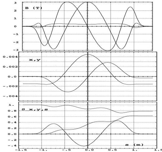
Figure 5: From top to bottom: field component, x and y coordinates, and spin components, at traversal of the cryogenic snake.
