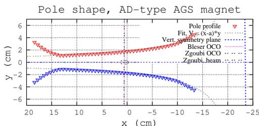
Figure 3: Pole profile in the OPERA model of AGS AF-type dipole. Machine center is to the left, virtual multipole — vertical symmetry plane is to the right at  $x \approx -23$  cm. (A second profile is of D-type, reversed gap shape wrt. the beam axis, it has been submitted to similar treatment.)
