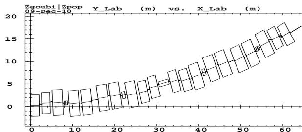
Figure 4: AGS super-period in Zgoubi. The origin of the super-period is at (0,0) on the “Zgoubi OCO line”.
