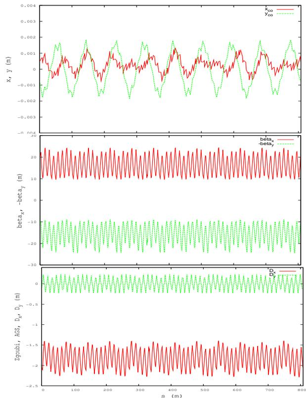
Figure 6: From top to bottom: H and V closed orbits, optical functions and dispersion.
