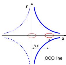
Figure 2: Off-centering of the beam (onto the OCO) in the multipole model.
