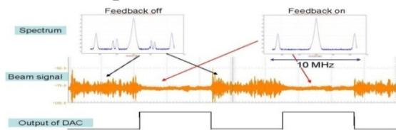
Figure 4: The horizontal betatron sidebands of beam in June 2008.
