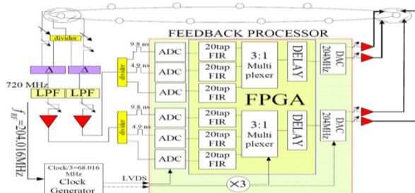
Figure 3: Overview of the HLS digital transverse Bunch-by-Bunch feedback system.
