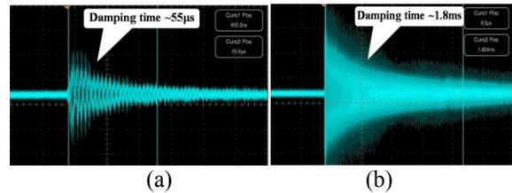
Figure 5: The damping time due to injection bump excitation was decreased by feedback system.
