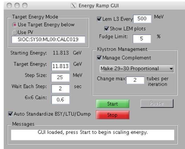
Figure 2: Energy Ramp GUI main screen.
