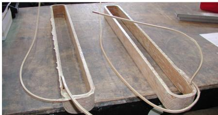
Figure 3: Kicker magnet copper coils.
