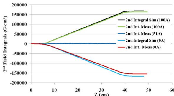
Figure 7: Measured and simulated 2<sup>nd</sup> field integrals at 0-A, 51-A, and 100-A correction currents.
