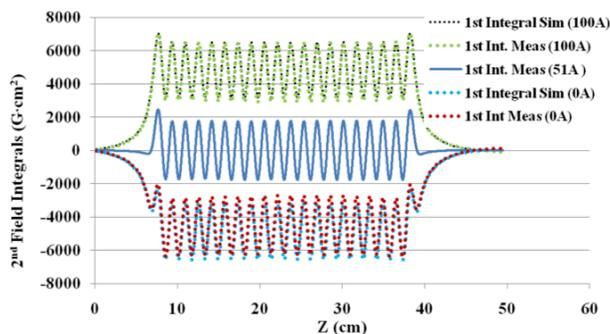
Figure 6: Measured and simulated 1<sup>st</sup> field integrals at 0-A, 51-A, and 100-A correction currents.
