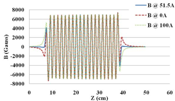
Figure 5: Field plots showing the effect of end-field correction currents at 0 A, 51.5 A, and 100 A.
