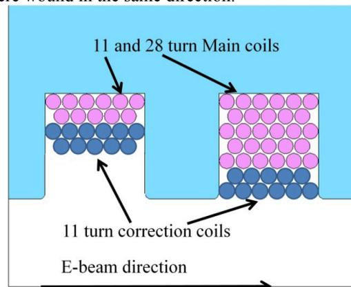
Figure 2: Winding configuration of the last two coil packs of one core. The magenta circles denote the main coils, and the dark blue circles the correction coils. The lighter blue depicts the steel core and poles.
