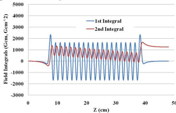
Figure 4: 1<sup>st</sup> and 2<sup>nd</sup> field integrals simulated with the Opera 2D computer code. Correction current was 51 A.
