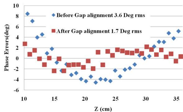
Figure 8: Phase errors before and after alignment of the gap, which corrected a small taper from end to end. Measured at 500 A with 51.5-A correction current.
