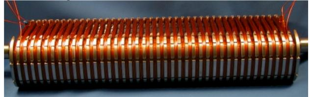
Figure 1: A single SCU0 core after completion of all winding and before potting with epoxy.
