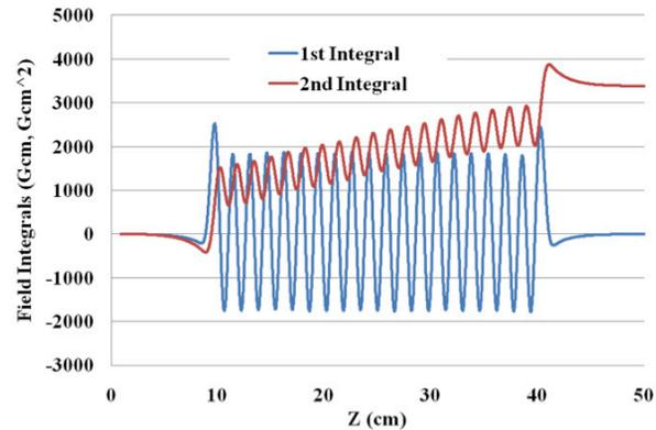
Figure 3: 1<sup>st</sup> and 2<sup>nd</sup> field integrals from measured Hall probe data from Fig. 5 with 51.5-A correction current.
