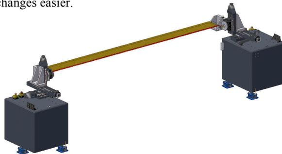
Figure 2: IFMS with the 4-m moving coil G10 board.
