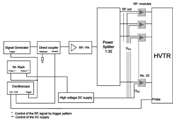
Figure 2: Schematic of the experimental measurement set-up.
