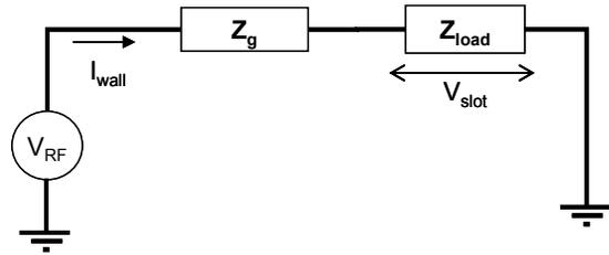
Figure 5: Equivalent circuit as seen from one module.
