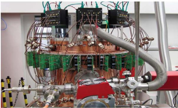
Figure 1: The  $\lambda/4$  resonator with 32 of 64 modules integrated.
