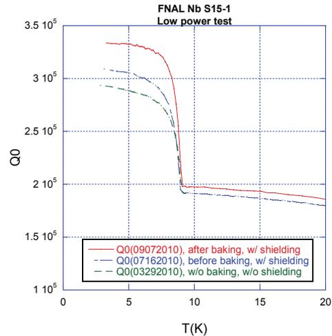
Figure 2<Low power test, FNAL small grain Nb0
