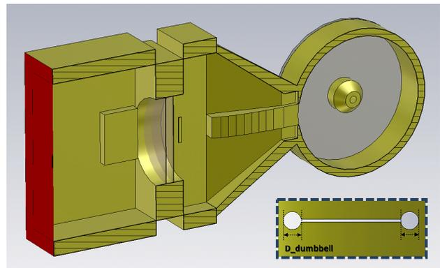
Figure 1: 3-D EM model on assembly of DTL tank cell, waveguide iris taper transition and WG window.
