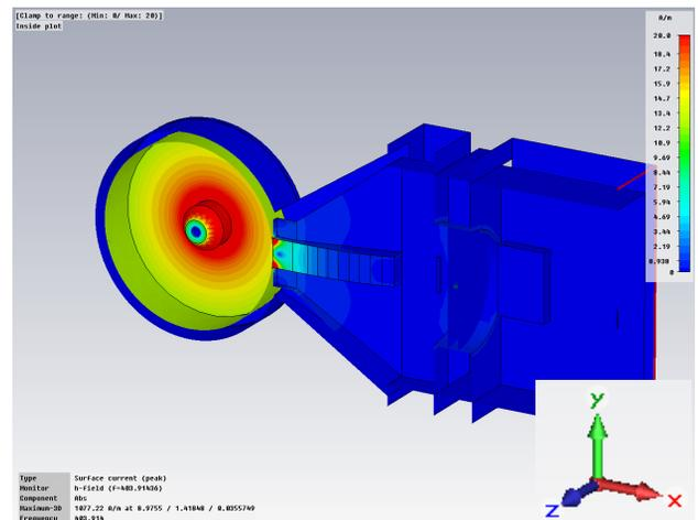
Figure 5: Surface current density plot of DTL/IRIS/Window model at resonant frequency (403.914MHz).
