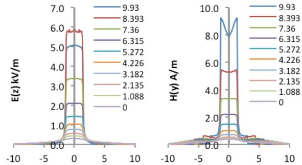
Figure 4: E(z) and H(y) field plots at each cross-section of ridged waveguide taper transition. Abscissas are transverse directions (y in inches) in model at  $z=0$ . Each curve represents distance (x) approaching to slot on DTL tank.
