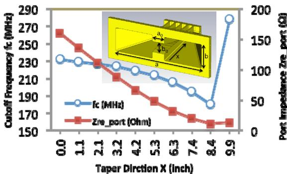
Figure 2: Double-ridge waveguide iris transition model and its cross-sectional port properties (cutoff frequency  $f_c$ , port impedance  $Z_{re\_port}$ ). Each point is based on CST model of waveguide with cross-section along x direction.
