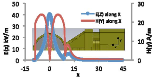
Figure 3: E(z) and H(y) field plots along the RF propagation axis (x-direction,  $y=z=0$ ). Beam axis (z-direction at  $x=y=0$ ), drift tube center has maximum E and minimum H field. E field drops rapidly at the coupling slot interface.
