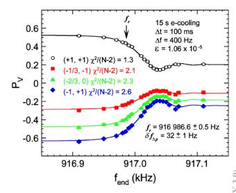
Figure 4: Measured 1.85 GeV/c deuteron vector polarizations plotted vs rf-solenoid end frequency  $f_{end}$ . Its ramp time  $\Delta t$  was 100 ms; its frequency range  $\Delta f$  was 400 Hz, and its  $\varepsilon$  was  $1.06 \times 10^{-5}$ . Electron cooling was on for 15 s. The curves are the Chao formalism fits giving the values of the resonance frequency  $f_r$  and of the Gaussian  $\delta f_{\Delta p}$  indicated in the plot.
