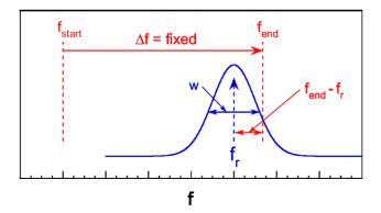
Figure 3: Schematic of the Chao formalism test. The rf solenoid's frequency  $f_{rf}$  was ramped, by a fixed range  $\Delta f$ , for different distances between the ramp's end frequency  $f_{end}$  and the resonance's center  $f_r$ . The curve shows the resonance with a total (FWHM) width w.
