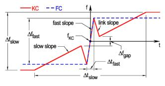
Figure 6: Kondratenko Crossing (KC) [solid line] and Fast Crossing (FC) [dashed line] patterns defining the parameters  $\Delta f_{fast}$ ,  $\Delta t_{fast}$ ,  $\Delta f_{slow}$ , and  $\Delta t_{slow}$ . The KC and FC patterns are both centered at  $f_{KC}$ .
