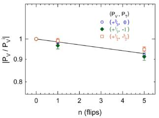
Figure 2: The measured vector deuteron polarization ratios at 1.85 GeV/*c* are plotted against the number of frequency sweeps. The rf dipole's frequency ramp time  $\Delta t$  was 60 s; its frequency half-range  $\Delta f/2$  was 75 Hz, and its  $\int B \cdot dl$  was 0.60 T·mm rms. The line is a fit using Eq. (5).
