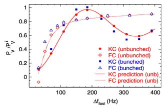
Figure 8: Measured 1.85 GeV/c deuteron  $P_V/P_V^i$ , averaged for all nonzero spin states, plotted vs fast frequency ramp range  $\Delta f_{fast}$ .
