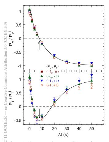
Figure 1: The measured vector and tensor deuteron polarization ratios at 1.85 GeV/*c* are plotted against the rf dipole ramp time  $\Delta t$ . The rf dipole's frequency half-range  $\Delta f/2$  was 100 Hz, and its  $\int B \cdot dl$  was 0.54 T·mm rms. The curves are fits of the vector and tensor data using Eqs. (3) and (4), respectively.
