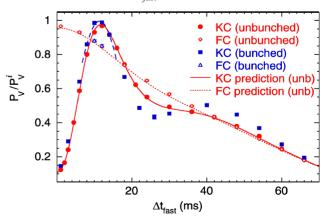
Figure 9: Measured 1.85 GeV/c deuteron  $P_V/P_V^i$ , averaged for all nonzero spin states, plotted vs fast frequency ramp time  $\Delta t_{fast}$ .
