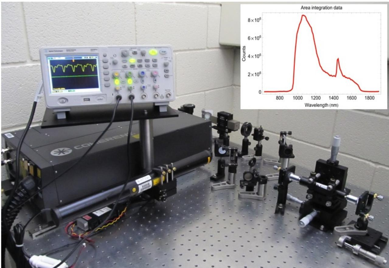
Figure 1: The set-up of 80-MHz Ti:sapphire oscillator and a PCF-800 commercial photonic crystal fiber device was used to generate the supercontinuum. The spectrum (insert) was measured using a Jobin-Yvon MicroHR spectrometer and a Xenics XS-1670 InGaAs camera.
