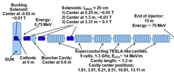
Figure 1: Schematic of the injector
