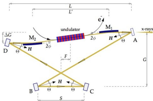
Figure 1: An X-ray FEL oscillator with a 4-crystal cavity.
