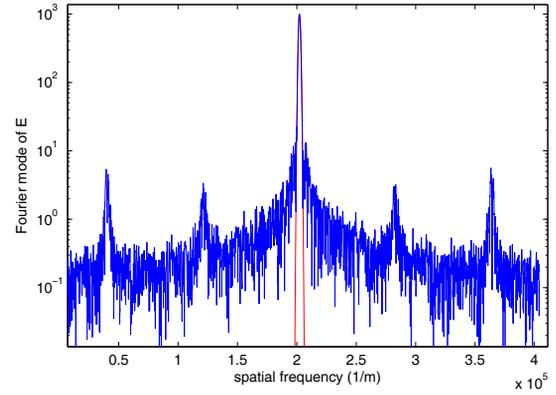
Figure 3: Fourier mode profile of  $|E|$  in  $k$  space at  $M_1$  (in log scale). Red line is incoming Gaussian beam and blue line is perturbed outgoing beam.
