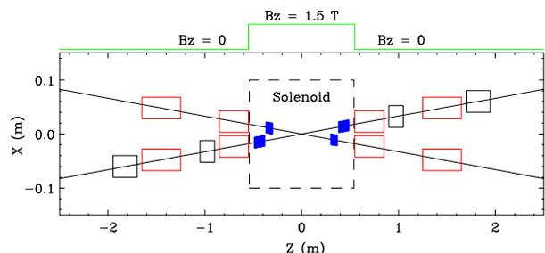
Figure 2: Effective hard-edge detector solenoid near IP.
