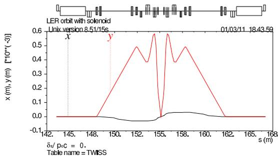
Figure 5: Corrected orbit in the LER IR.
