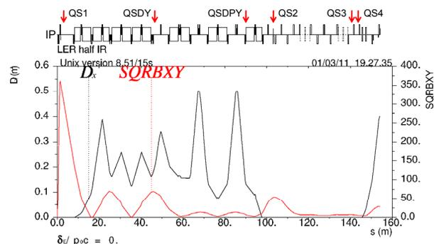
Figure 4: LER skew quadrupoles in half-IR. Plotted functions are dispersion and  $\sqrt{\beta_x/\beta_y}$ .
