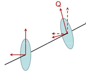
Figure 3: Quadrupole rotation to align with beam rotation.
