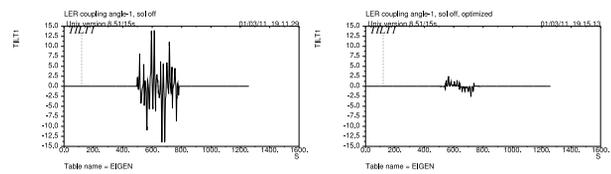
Figure 8: LER beam tilt angle (deg) for mode 1 with solenoid off. Left - original QD0P rotation, right - optimal QD0P rotation.
