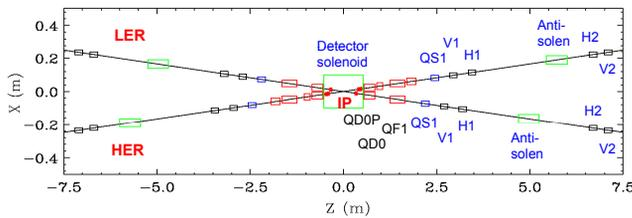
Figure 6: Solenoid correctors within  $\pm 7.5$  m of IP.
