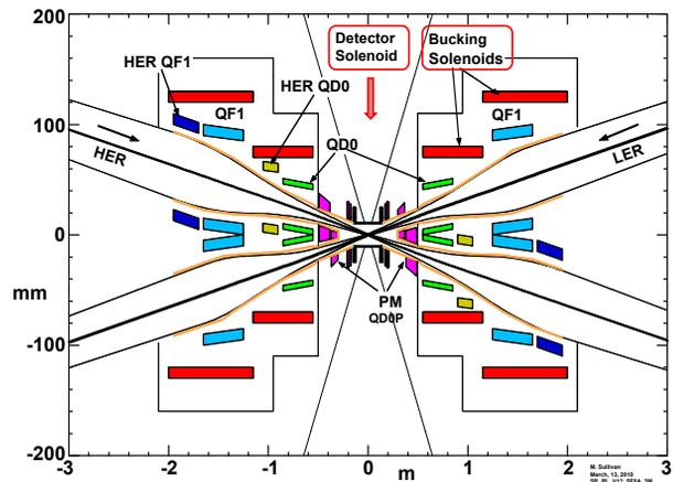
Figure 1: IR layout with detector and bucking solenoids.
