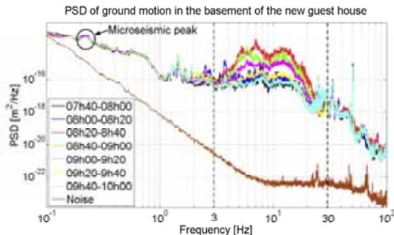
Figure 2: Vertical ground motion at the INFN/LNF site
