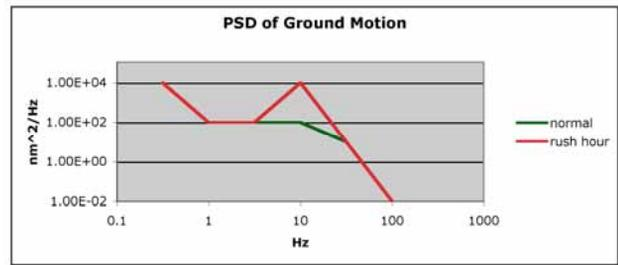
Figure 4: Idealized ground motion spectrum for modeling
