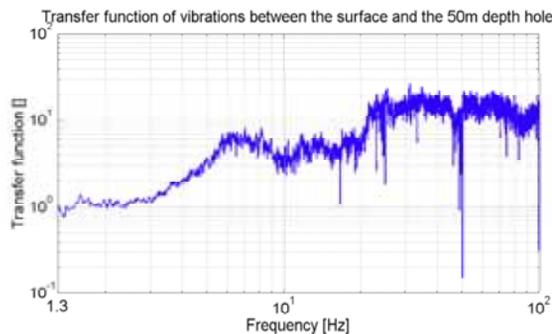
Figure 3: Attenuation of vertical motion with depth
