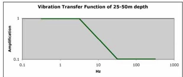
Figure 5: Idealized transfer function due to depth
