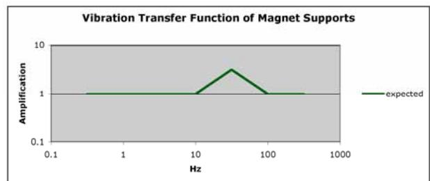
Figure 6: Vibrational behavior of normal magnet supports
