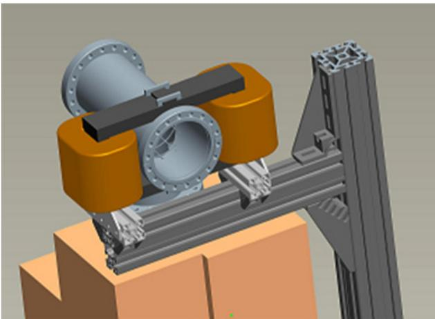
Figure 7: Dipole corrector mounted on its stand. Also shown is the vacuum-T where the magnet is located.
