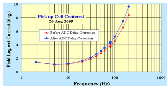
Figure 4: Measured frequency response of the prototype laminated yoke corrector magnet.
