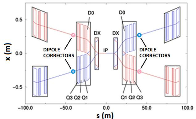
Figure 1: Schematic view of the RHIC “6 o’clock” interaction region. The circles indicate the approximate locations of the corrector magnets close to the cryostats.
