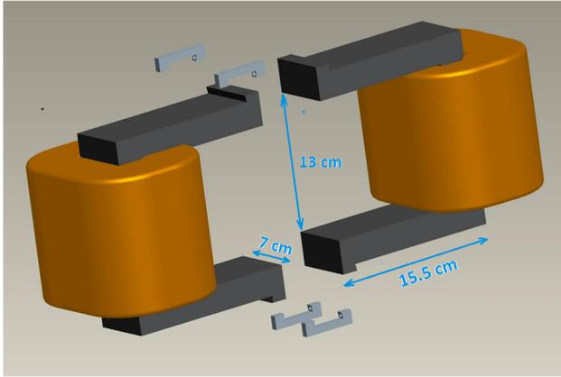
Figure 2: Drawing of the two halves of one of the corrector dipoles and the clamps used in their assembly designed so as to avoid vacuum system disruptions during installation.
