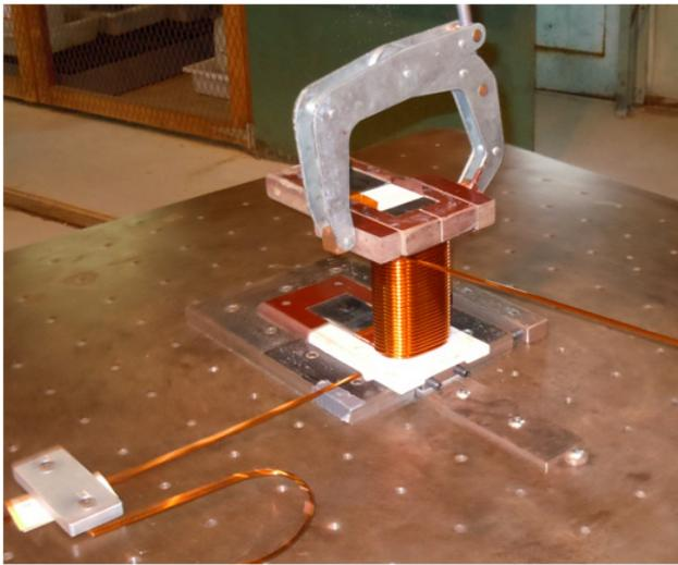
Figure 5: Rotating table arrangement for coil winding.
