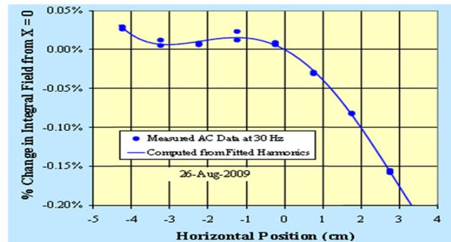
Figure 3: Example of measured integrated field variations as function of distance from the nominal beam axis, obtained with a 0.61 m long flat coil and 30 Hz field excitation in this case.
