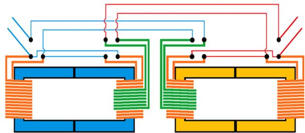
Figure 8: Schematic diagram of the connections for a pair of corrector dipoles mounted close to each other on the “blue” and “yellow” rings. The green windings are the compensation coils connected in series with the main coils of the opposite magnet.
