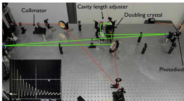
Figure 4: Initial bench top test of the RING resonator. An injected 1064  $\mu\text{m}$  laser beam (red line) generates 2<sup>nd</sup> harmonic (green line), which is trapped inside the cavity.
