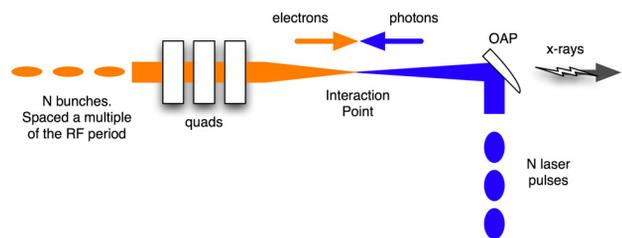
Figure 1: A conceptual diagram of the multi-bunch ICS.
