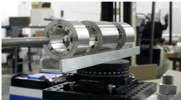
Figure 3: PMQ triplet on the test stand. The 3D Hall probe enables 3D field map measurements, which can be imported into ELEGANT for beam dynamics simulations.
