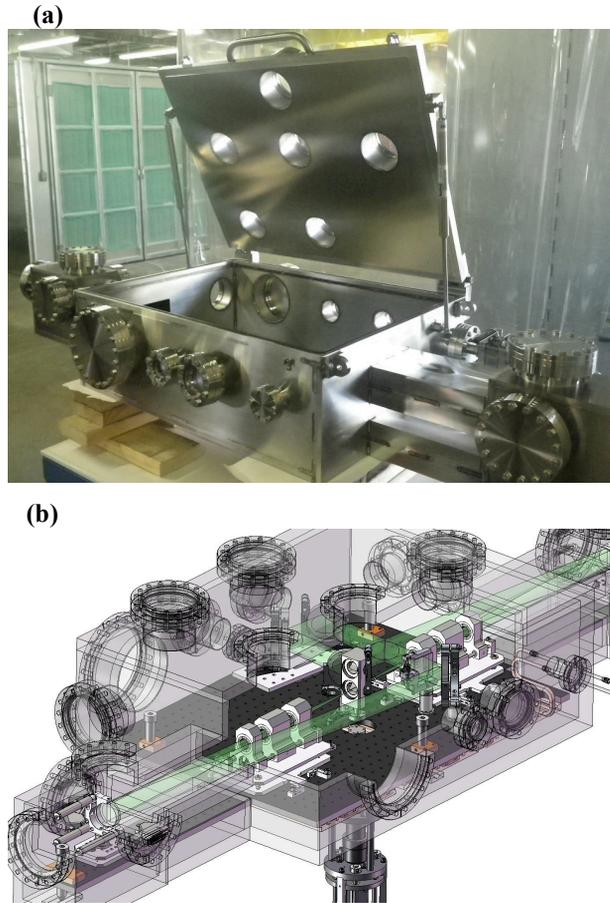
Figure 2: A photograph of the ICS interaction chamber prior to initial UHV test (a); and a CAD model of a full ICS assembly (b), showing vacuum chamber, diagnostics, laser beam envelope, PMQs and RING optics.
