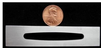
Figure 4: SCU vacuum chamber extrusion cross section.
