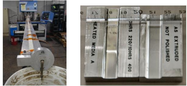
Figure 3: Abrasive flow polishing process and samples before and after polishing
