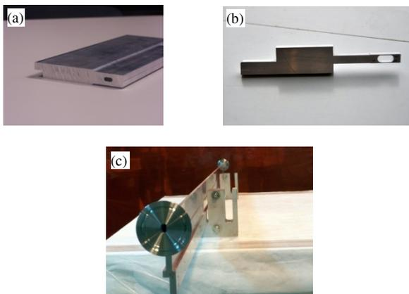
Figure 2: (a) Extrusion section; (b) machined chamber cross-section; (c) welded vacuum chamber prepared for cleaning.
