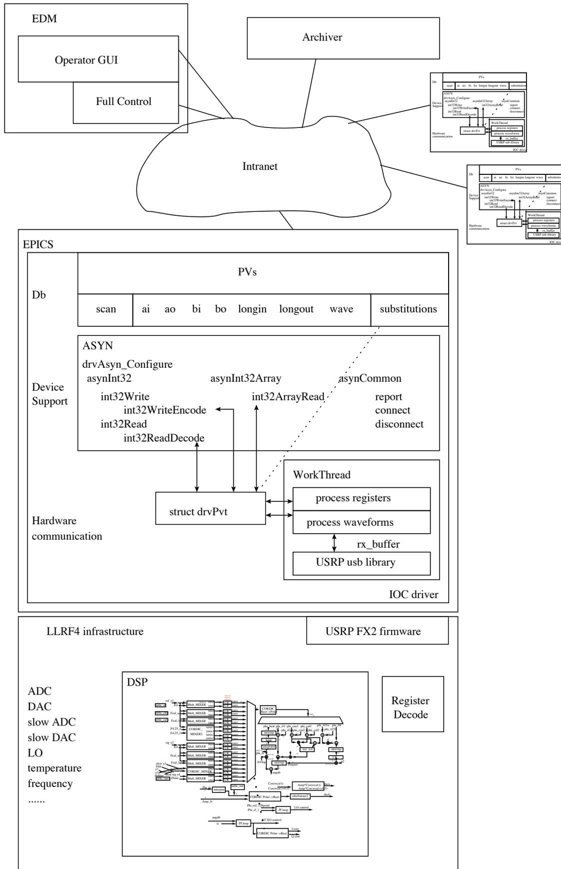
Figure 2: LCLS Berkeley femto-second timing and synchronization system Software and firmware architecture
