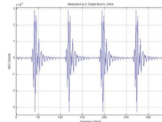
Fig. 1: Measured ALS Single Bunch
