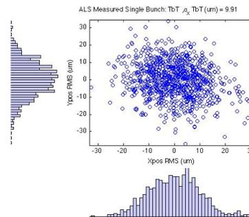
Fig. 2: Single Bunch TbT Scatter-Histogram
