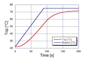
Figure 3: Simulation results (ANSYS). Lower curve (red) represents the temperature of the top surface.
