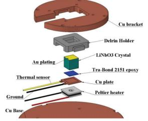
Figure 2: Holder assembly for optimized thermal transmission.
