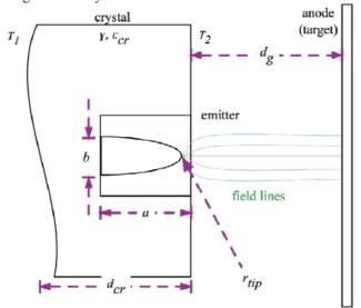
Figure 1: A cross-section of an emitter tip, showing an anode, and (conceptual) field lines.
