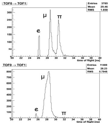
Figure 3: TOF distributions for 300 MeV/c  $\pi$  (top) and 200 MeV/c  $\mu$  (bottom) beam with separation of  $e^+$ ,  $\mu^+$ ,  $\pi^+$ .
