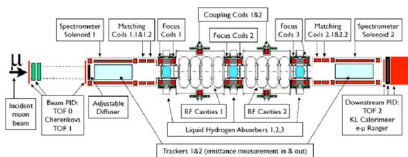
Figure 1: Schematic of MICE cooling channel.
