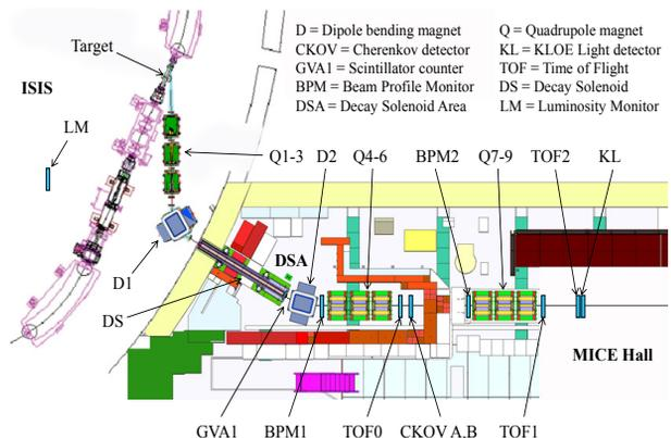
Figure 2: The MICE upstream beamline in 2010 configuration.
