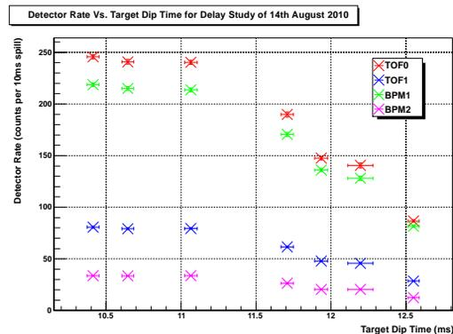
Figure 5: Particle rate in several beamline detectors as a function of target dip timing (nominal at 11.7 ms).
