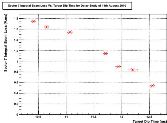
Figure 7: ISIS integrated beam loss vs. target dip timing with nominal dip time at 11.7 ms.
