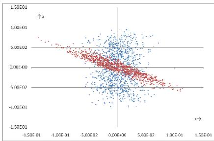
Figure 3 Initial (blue) and final (red) distribution in horizontal phase space for 1 Twin Helix cell.
