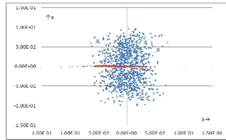
Figure 5: Initial (blue) and final (red) distribution in horizontal phase space for a series of 50 Twin Helix cells.
