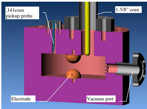
Figure 3: Cutaway view of the 1.3 GHz Cavity.
