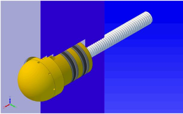
Figure 5: Cut-away view of moveable electrode design.
