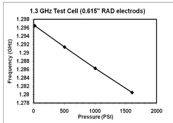
Figure 4: Resonant Frequency Varies with Pressure
