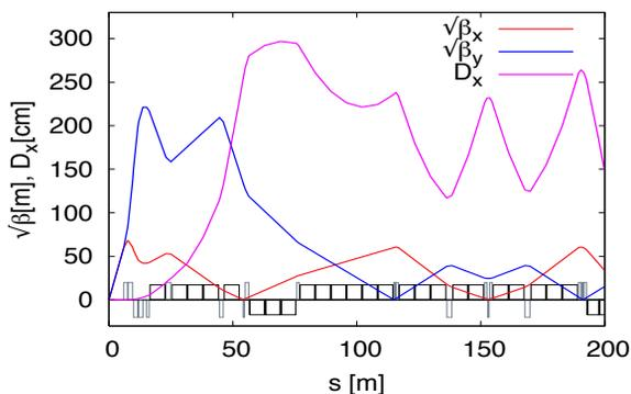
Figure 1: IR layout and Twiss functions.
