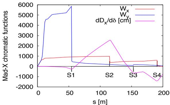
Figure 2: IR MAD-X chromatic functions,  $W_z = \sqrt{A_z^2 + B_z^2}$ , and sextupole locations. The sextupole S3 at 150 m corrects  $dD_x/d\delta$ .
