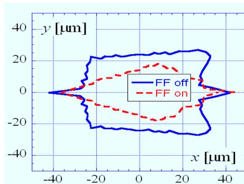
Figure 3: 1000 turns DA w/o (blue contour) and with (red) fringe fields.
