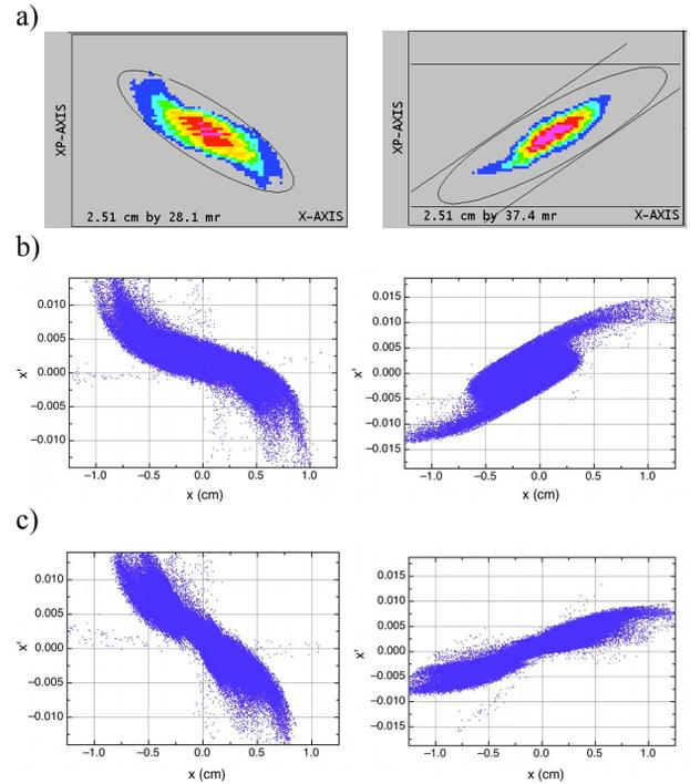
Figure 2: Comparison of measured and simulation results at (left) TBEM3 and (right) TDEM1 beam emittance stations: (a) measurements, (b) simulation with current  $I = 15$  mA, (c) simulation with current  $I = 0$ .
