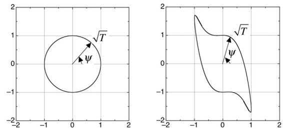
Figure 4. Distortion of beam emittance due to aberrations, Eq. (7): (left) nonlinear perturbation  $\nu = 0$ , (right)  $\nu = 1.6$ .
