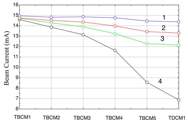
Figure 5. Beam transmission through LEBT as a function of vacuum conditions: (1)  $4.6 \cdot 10^{-7}$  Torr, (2)  $7.4 \cdot 10^{-6}$  Torr, (3)  $1.3 \cdot 10^{-5}$  Torr, (4)  $4.9 \cdot 10^{-5}$  Torr.
