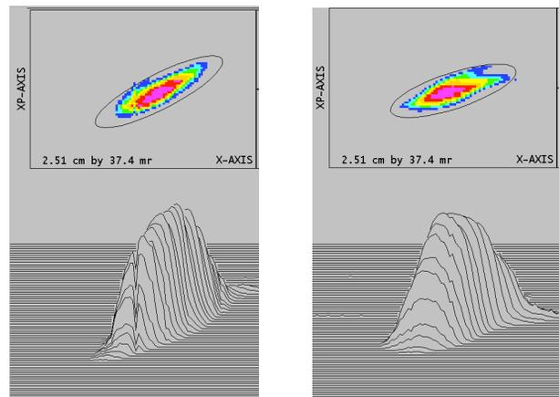
Figure 6. TDEM1 emittance scan with (left) nominal vacuum of  $7 \cdot 10^{-7}$  Torr and (right) with vacuum of  $3 \cdot 10^{-5}$  Torr.
