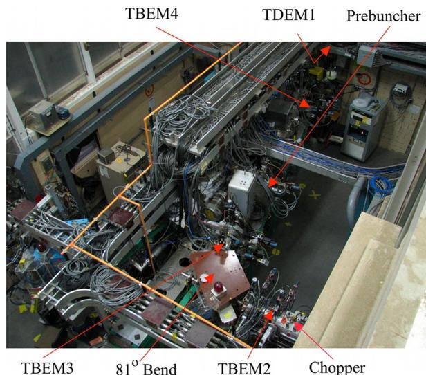
Figure 1. Layout of H<sup>-</sup> Low Energy Beam Transport of LANSCE.
