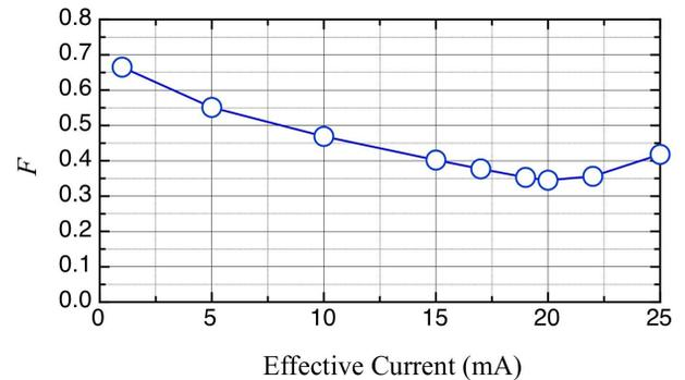
Figure 3. TRACE mismatch factor  $F$  as a function of beam current in beam drift between TBEM3 and TBEM4.
