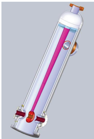
Figure 2: Cut away 3D view of the low beta quarter wave resonator. The overall height is about 85 cm.
