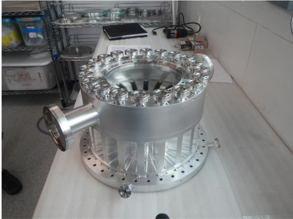
Figure 8: A component of the funneling polarized electron gun. Laser input ports are shown on top.
