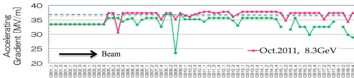
Figure 5: Acceleration electric-field gradients of all the C-band units along the SACLA accelerator. The electric-field gradients of almost all the C-band units after BC3 reach values of more than 37 MV/m. The red line with the solid triangle dots shows the case at a beam energy of 8.3 GeV; the green line with the solid round dots shows the case of 7 GeV. The blue dotted line is a reference value of 37 MV/m.
