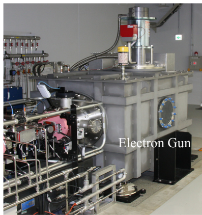
Figure 2: Outlook of the 500 kV, CeB 6 thermionic electron gun.
