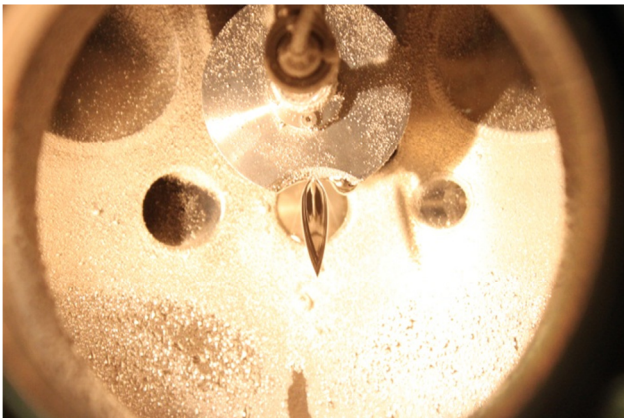
Figure 2: Liquid lithium film established at ANL.
