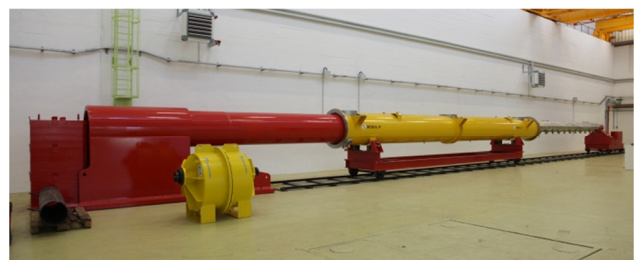
Figure 3: Vacuum vessel and cold mass on the cantilever
