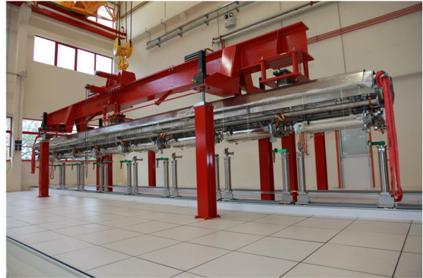
Figure 5: PXFEL2_2 cold mass and string hooked to the girder in the Roll-Out area
