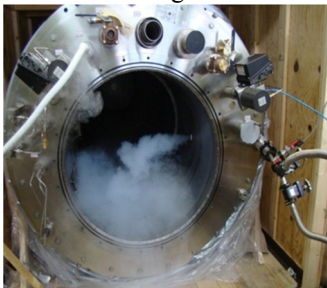
Figure 9. VTS Cryostat under cold shock testing
