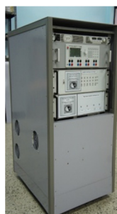
Figure 10. 500 W Solid State RF system for VTS
